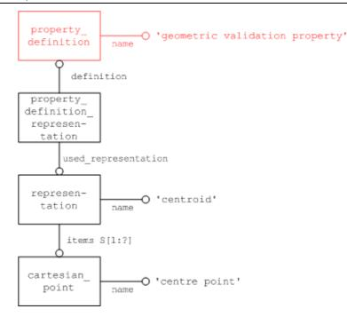
Figure 5: Geometric Validation Property "Centroid"
