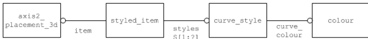
Figure 10: Coloring an Axis Placement
