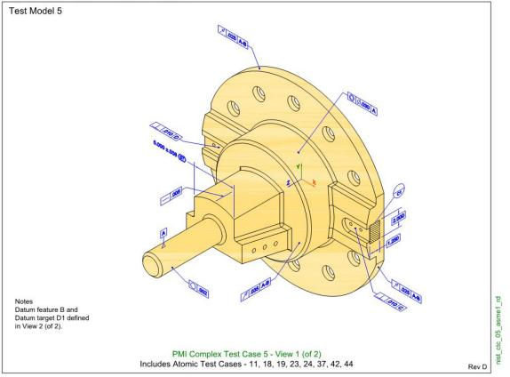
Figure 8: Illustration of the CTC-5 model used for the ASR test case
