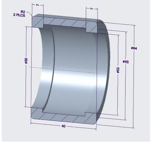
Figure 15: Illustration of PID\_3 Test Case
