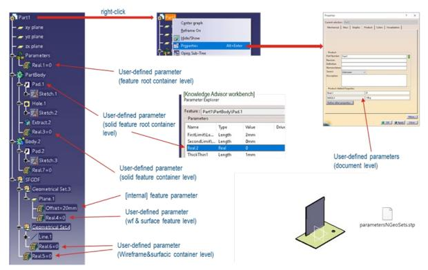
Figure 12: Overview on Parameters and Properties defined in the CATIA model
